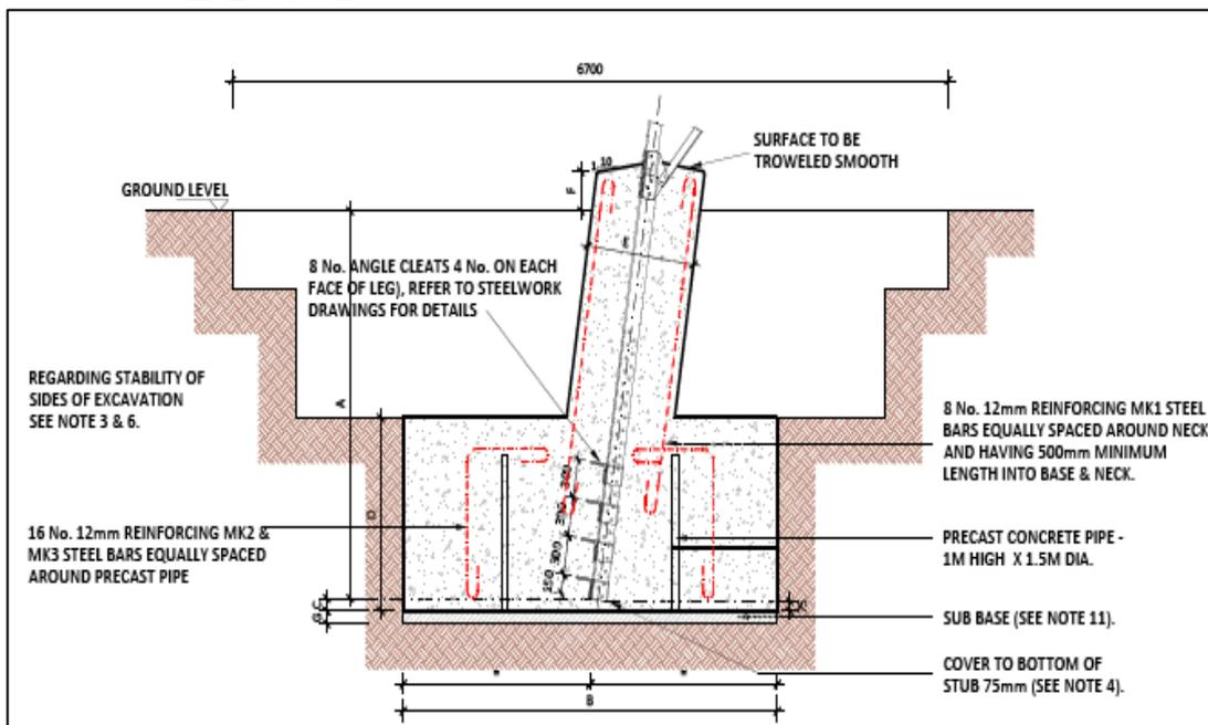
Plate 4-11 Steel lattice tower foundation
