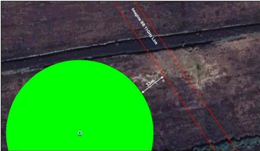
**Figure 14. Proposed Turbine relative to Imagine BB Radio Link – Plan View**
